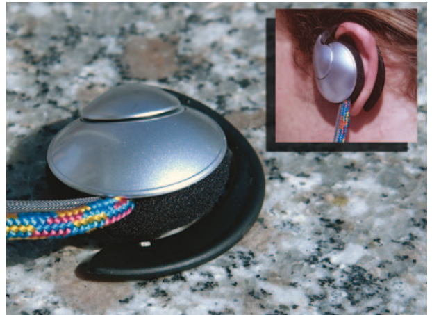
Figure 1: Heart rate sensor integrated in a commercial earphone.
