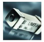
SCHURTER's Universal Modular fuse, UMT-H, offers a 1500 A breaking capacity at rated voltages of 277 VAC / 250 VDC. The compact, high performance fuse now has VDE approval in addition to UL approval. This time-lag fuse provides overcurrent and short circuit protection in various industrial control applications, including intrinsically safe applications.
