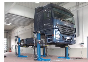
Mobile Column Lift for Heavy Vehicles. Large picture: Lifting a truck. Two small pictures: Handling and operational status at a bus wheel
