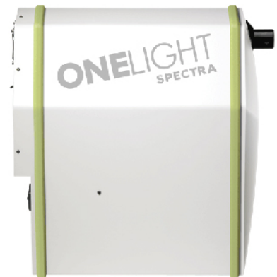
Profile view of the OneLight Spectra Spectrally Programmable Light Engine (SPLE).
