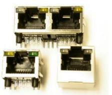
All LEDs run at 2.1 volts nominal and consume 20 milliamps. Many custom LED color combinations are available, as well as the selective loading of contacts, custom contact plating, and special shielding. Right angle jacks can be made with a larger housing that allows for the incorporation of customer-specified filter components.
