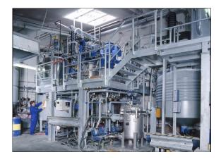
ROWA Lack has installed new vacuum dissolvers at their Seevetal site, thus investing in modern production standards. The identical configuration of these vacuum dissolvers guarantees a comparable quality picture in all conceivable trial and production phases. With the new dissolvers, only closed processors are used in the solvent sector. This enables ROWA Lack to comply with all emission-limiting requirements of the VOC regulation and reduces even further the very minimal environmental
