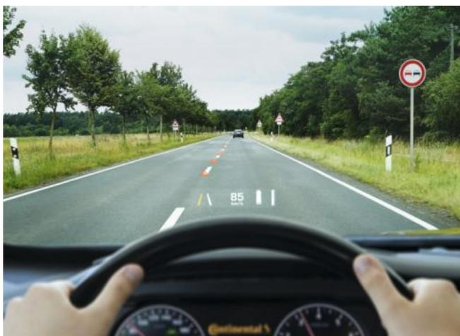
Three applications are implemented in the AR-HUD demo vehicle as examples: Lane Departure Warning (LDW), Adaptive Cruise Control (ACC), and navigation.
