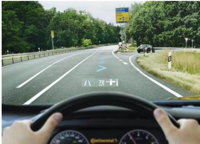
The Augmented Reality Head-up Display moves virtual information directly into the driver's line of sight. The AR-HUD inserts full-color graphics into the real road view at a distance of 7.5 meters.
