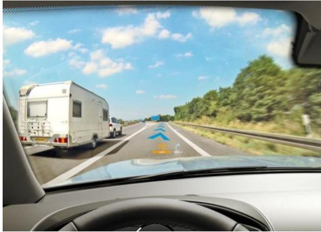
With the Augmented Reality Head-up Display the View of the road and the extended horizon of a vehicle will blend into one in the future
