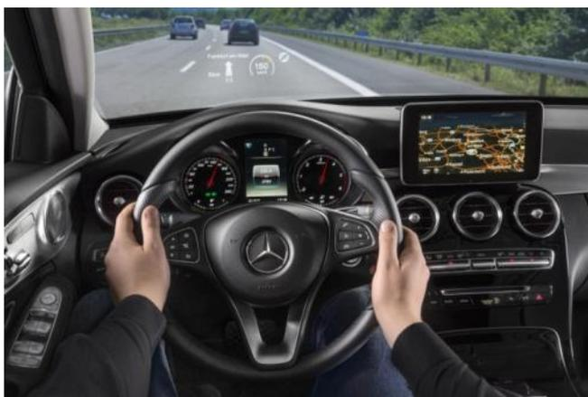
In its current version, an HUD is an outstanding information filter. It moves a minimal amount of carefully selected information into the driver's line of vision
