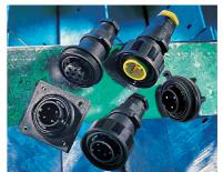
This well known, long standing range of IP68 rated connectors comprises 7 body styles, including flex, flex in-line, front and rear panel, PCB, bulkhead and flange mounting and are available in 2, 3, 4, 6, 7, 9, 12 and 25 poles. Ratings range from 1A, 50V to 12A, 250V.
