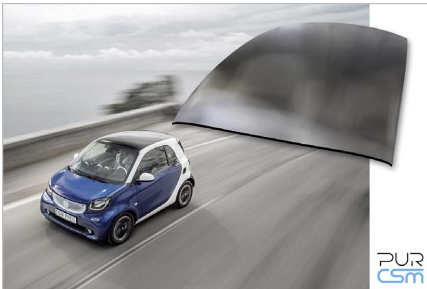
Material mix of polyurethane, glass fibre and paper honeycomb: lightweight roof for the smart "fortwo"
