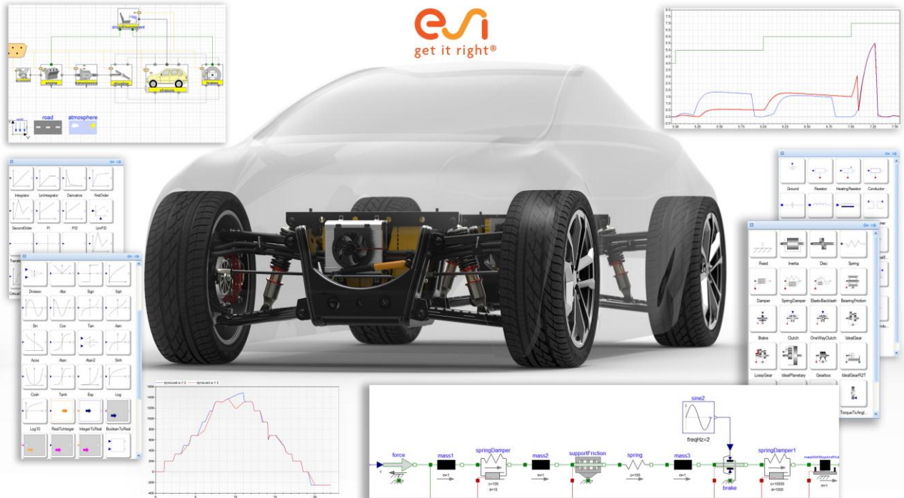
Image: Example of 0D-1D systems modeling in Visual-Environment illustrating how ESI-Xplorer can assist the design and development of architecture, systems, parts and controls for automotive powertrains.
