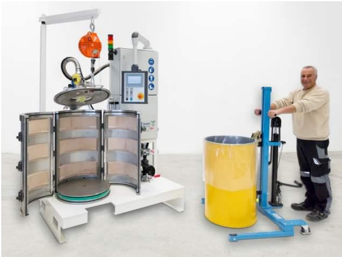
Figure 2: With the new TAVA 200 F semi-automatic vacuum station from Tartler, material manufacturers can fill 200 litre lidded drums with pasty and high-viscosity resins without any air pocket formation. The system can be easily designed for other container sizes too.
