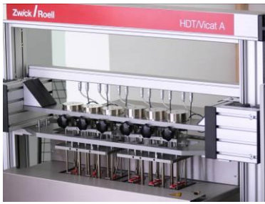
Fig. 1: HDT/Vicat-tester comprising 6 test stations
