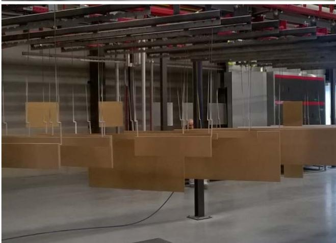
New flexible gascatalytic IR oven for kitchen front panels
