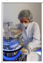
Pharmaceutical production: New pharmaceuticals are first manufactured on a smaller technical scale. During this process the later production conditions are simulated, and the manufacturing process and tablet composition are optimized. In addition, the tablets with active ingredients and the placebos (without active ingredients), which are both necessary for clinical studies, are produced.
