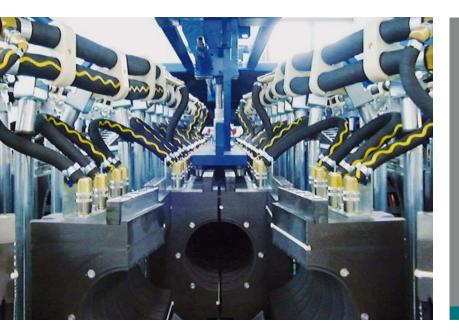
The semi-automatic QuickChange system for mould block change reduces your HD 250's setup and maintenance intervals by approx. 30%!
