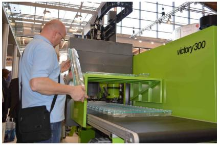
In an eight hour shift, without interruption, over 523 luminaire housings were injection moulded, foamed, and placed on a discharge belt for curing and further processing.
