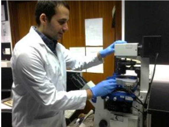
Faris Sinjab is a PhD student in the group of Dr Ioan Notingher is seen using the JPK NanoWizard® AFM system
