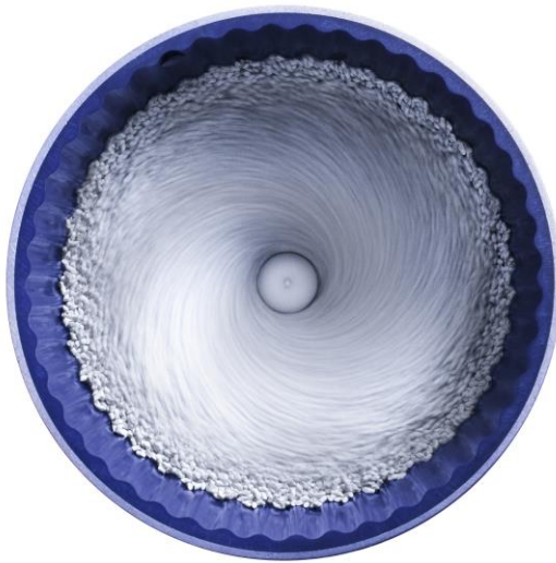
Deburring and rounding with Disc Finishing Technique
