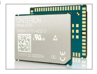
low and high-volume M2M devices with regard to reliability and efficiency. The module measures only 18.8 x 27.6 x 2.3mm and its outstanding performance and commonly used industrial interfaces such as USB, Serial and Digital Audio makes it the perfect choice for both Voice and Data Communications. The EHS5-E (900/2100 MHz) and EHS5-US (850/1900) enable global 3G coverage and will seamlessly fall back to Class 12 GPRS/EDGE when required.
