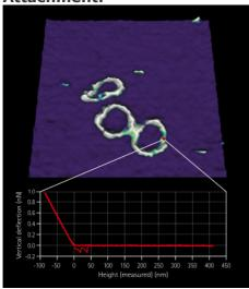
168 bp DNA nanorings on Poly-L-Ornithine protein layer in buffer solution and force distance curve at the marked point. Scan size: 80 x 80 nm. Z-range: 2.5 nm. Imaged in closed-loop. Sample courtesy of Dr Damian Ackermann, LIMES, University of Bonn, Germany.
