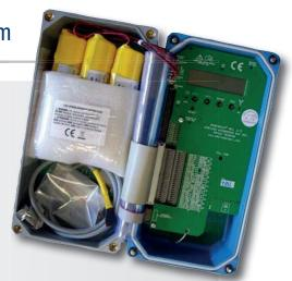
SensoBrick® is a complete and self-sufficient in-a-box monitoring solution. Its embedded temperature sensor for environment and substrate, biaxial inclinometer for pitch and roll, 3-axis accelerometer and seismic trigger monitors thermal-, seismic-, vibration- and settling-induced actions on buildings, infrastructures or industrial plants. Numerous additional input ports allow for integration of application specific sensors to form a modular system to cover your specific monitoring needs.
