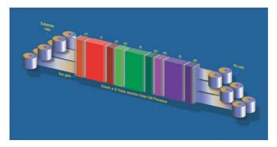
UNI-SOLAR® solar cells are made in a roll-to-roll vacuum deposition process on a continuous roll of stainless steel sheet. The result is a unique, flexible and lightweight cell. The solar cells are arranged in a series string and encapsulated in UV stabilized and weather-resistant polymers to form PV Laminates. The polymer encapsulation includes at the front side EVA and the fluoro-polymer ETFE (e.g. TEFZEL® from DuPont).
