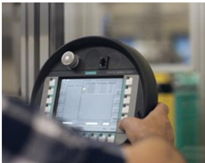
The Simatic Mobile Panel with editor interface uses the new performant G-Code interpreter to translate the taught contour programs in the Simotion D445 into high-dynamic, precise movements.
