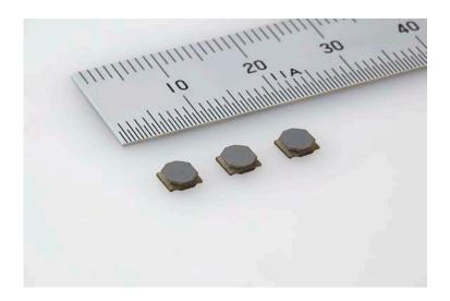
Tokyo, May 15, 2014 — TAIYO YUDEN CO., LTD. today announced the addition of eight items including the "MDMK4040T1R0MM" (4.0 x 4.0 x 1.2mm, the maximum height value), which has an approximately 20% reduced DC resistance than the company's previous product, to its metal core SMD power inductors (MCOIL<sup>TM</sup>, MD Series).
