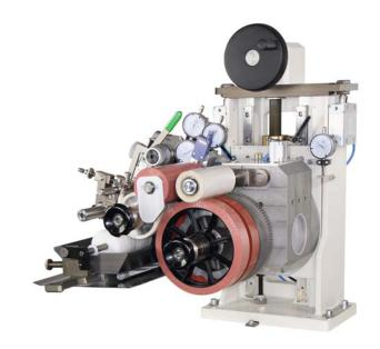
"RTI 21-150", Rotary built-in tampon printing unit
