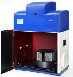
NightSHADE is equipped with a highly sensitive 1 Mpixel slow scan CCD camera cooled to an absolute temperature of -70 °C. This insures lowest background and highest sensitivity even when very long exposure times are required.
