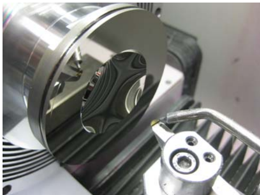
Image: view of inner machine space showing a workpiece with free-form surface being processed
