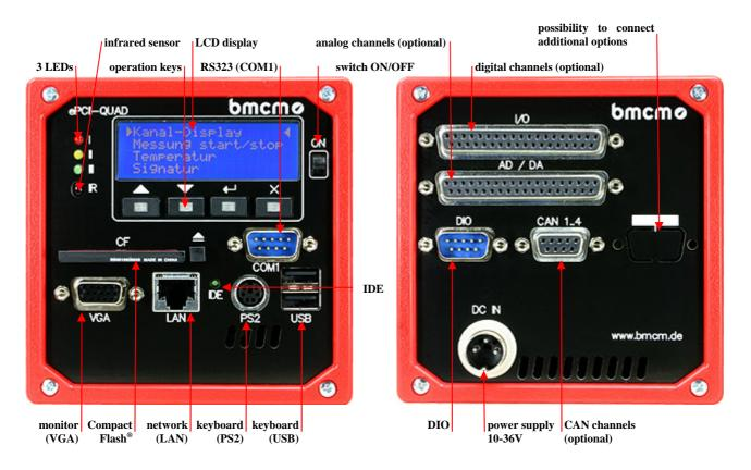
If the **ePCII-QUAD** is extended with additional PC/104 interface cards the corresponding Sub-D connectors can be mounted at the back of the device (see chapter 3.11). For pin assignment please see the relevant data sheet.
