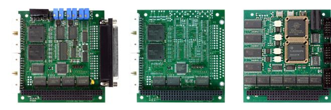
To record analog or digital signals a measuring card (e.g. PC104-AD12/16, PC104-PIO48) can be integrated in the **ePCII-QUAD** on request. To provide the **ePCII-QUAD** with additional CAN and COM interfaces, various interface cards are available. All extension cards are implemented in PC/104 standard.
