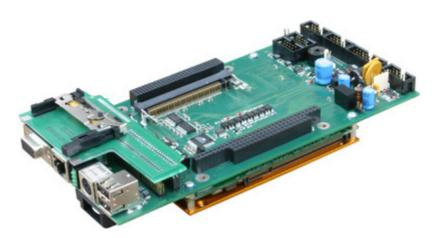
The integrated carrier board **ePCII-CB+LX800** is the central element of the **ePCII-QUAD**. Via various internal and external connections it is attached to the different components (CPU, display, keyboard, I/O cards), routes incoming signals and realizes basic PC functions (e.g. reset, basic supply by battery). A system connector in standard PC/104 technology allows for the connection of additional PC/104 cards (see chapter 4.4).
