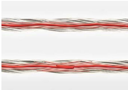
Structural representation of dual core yarns (top) and a properly spliced joint (bottom)
