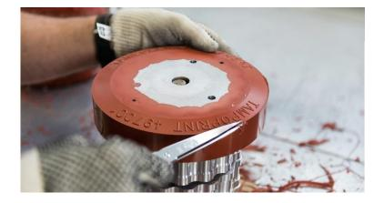
Finishing touches by hand on a CRS pad ring for rotation pad printing machines
