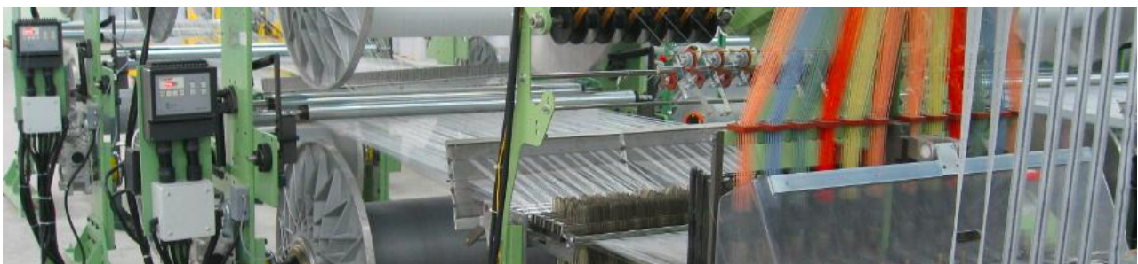
Beam rack for elastic tapes
