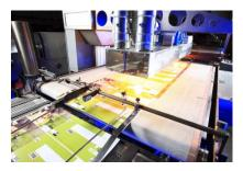
**Caption 1**. After retrofitting Heraeus carbon infrared (CIR) emitters in place of an NIR infrared print drying system, the Alito Color Group has been able to realise the full potential of its high speed print heads, by increasing sheet feed speeds to match the print speeds with no detriment to print quality. (Image: Heraeus Noblelight GmbH)
