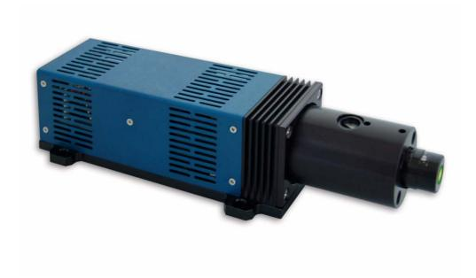
Green PowerLine structured light laser offers a thermoelectric system and fan that maintains a constant laser diode temperature, resulting in better wavelength, power, and pointing stabilities. The Green PowerLine design makes focusing even easier with the focus adjusting screw located directly on the body of the laser.
