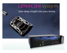
FOGALE nanotech's Low Coherence Interferometric Sensor (LISE) relies on the measurement technique of low coherence interferometry, also referred to as partial coherence interferometry. By comparing the optical paths in the glass with the optical path in an internal delay line, the system allows to measure the positions and thicknesses of glass layers and interlayer products.
