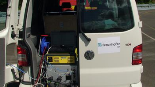
Picture 2: Mobile gas analytics tool of the Fraunhofer ICT, on site during an electric vehicle crash test
