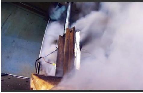
Picture 4: Gas release from a lithium-ion cell during an abuse test
