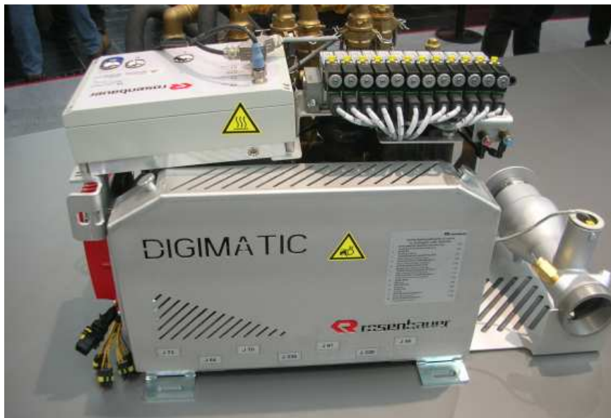
Fig. 2: The Rosenbauer DIGIMATIC42 pressurized foam mixing system is electrically driven with a controller and motor from the Nuremberg-based drive and automatization manufacturer Baumüller
