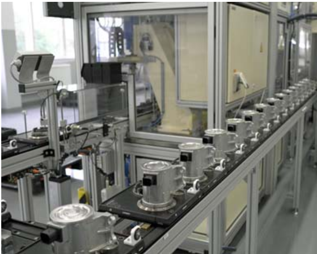
Photo 2 - Production of CWA 400 Pierburg Pump Technology at Hartha/Germany plant.
