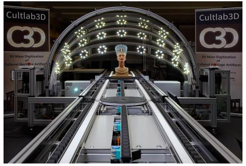
Image: From 11 to 14 November 2014 the researchers of Fraunhofer IGD test their 3D scanning system CultLab3D together with the Natural History Museum in Berlin. The aim is to explore the opportunities and challenges of digitizing natural and cultural goods quickly and efficiently. Here you see the scanning system with a replica of Nefertiti.
