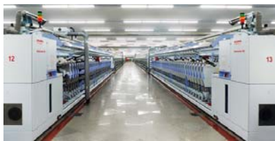
Zinser 351 directly linked to the Autoconer X5
