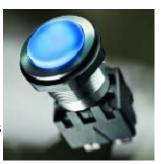
The new MSM LA CS ON/OFF stainless steel pushbutton switch from SCHURTER is equipped with an actuator made of durable ceramic. The same ceramic is already being used to manufacture the previously introduced MSM CS momentary action switches. The material resists scratches and abrasive chemicals as well as impacts; it can also be labeled with highly endurable legends.
