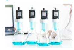
Mount the drive onto the cartridge and install it on the shake flask. LIS will now automatically run your feeding profile.
