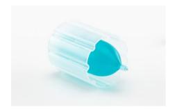
The cartridge is a single use container with the shape of a lid for shake flasks. It fits on all shake flasks that are normally sealed with a metal cap. The cartridge comes sterile packed and is for one time use only.
