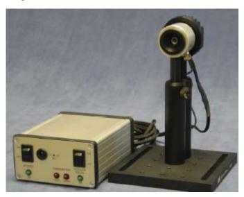
The STEP-45 or STEP-49 includes the STEP-Controller module. The controller provides power and temperate control and the analog detector output.
