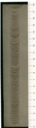
Fig. 3: Hot wire narrow gap weld. One pass per layer. Wall thickness 180 mm, base material: low alloy steel P91. Foto: Polysoude Photo: Polysoude
