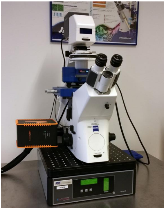
The combined Abberior STEDYCON and JPK NanoWizard® AFM setup at the JPK headquarters in Berlin.
