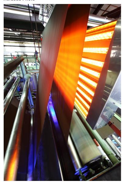
Fast response medium wave infrared emitters dry coatings quickly and safely.
