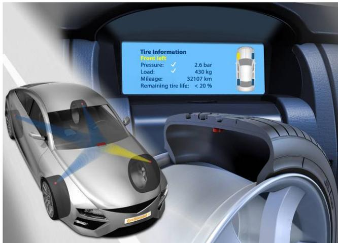
Intelligent tire sensors, which are integrated into the tires, deliver information about the current tire distortion of the rolling tire.
