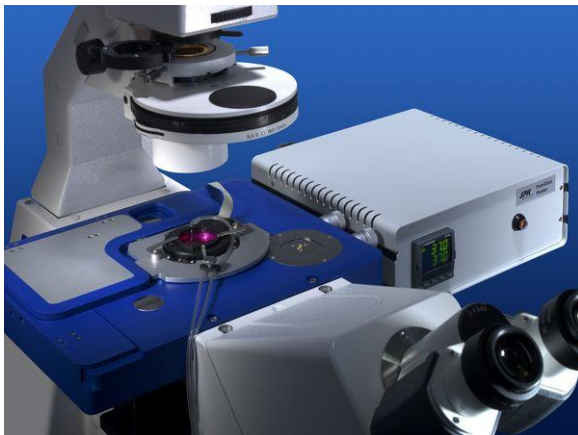
JPK's Petri dish heater mounted on a Zeiss microscope for live cell imaging studies
