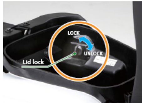
■ Connector lid lock function
